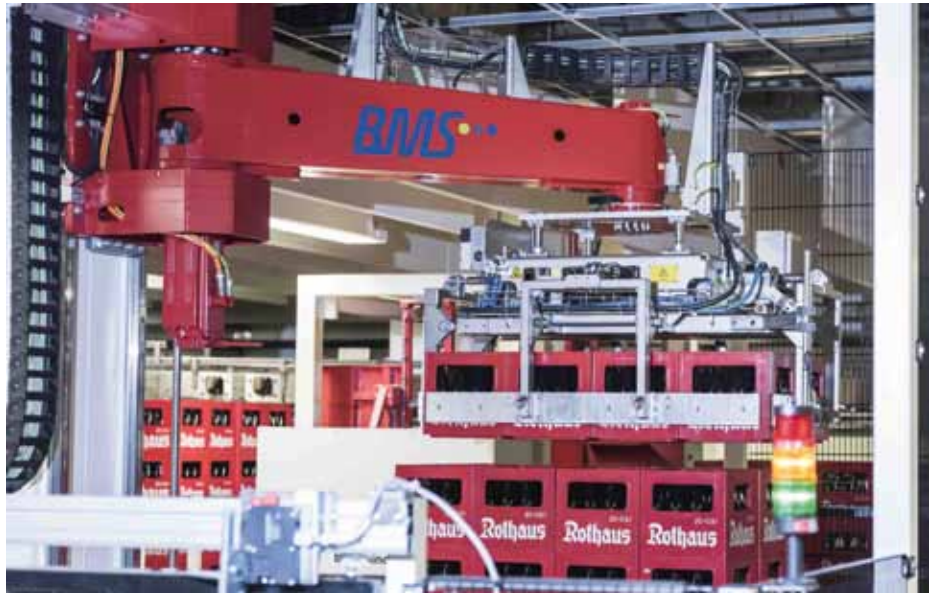
Rothaus chose a column-type palletiser for both the loader and the unloader
